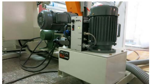
Controller Series 49 is installed on TOUGU DENKI Hydraulic Actuator directly
